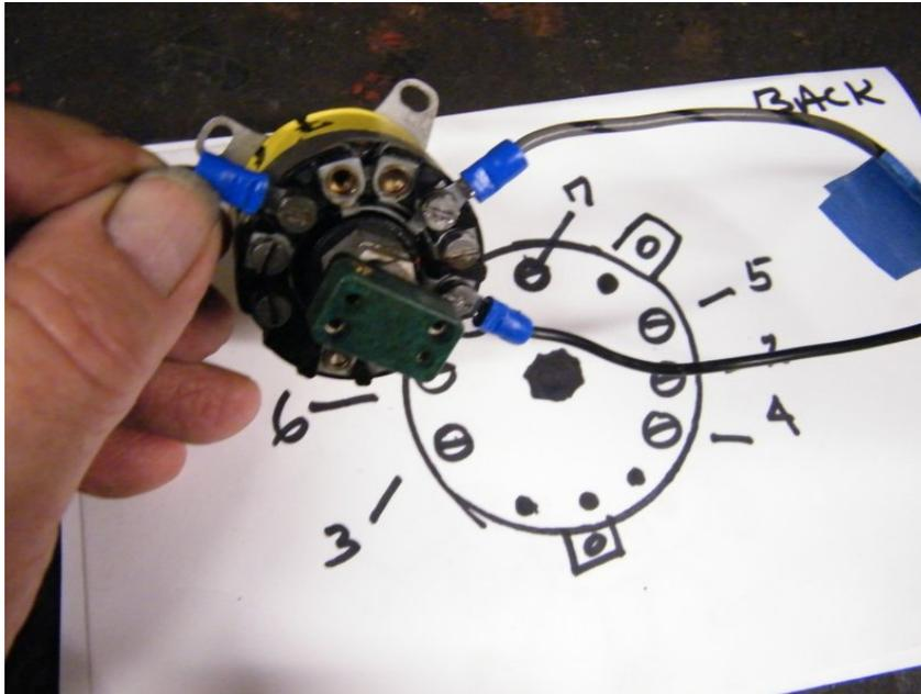
At the side of the switch are numbers stamped into the metal case, identifying each terminal, not in sequential order.
