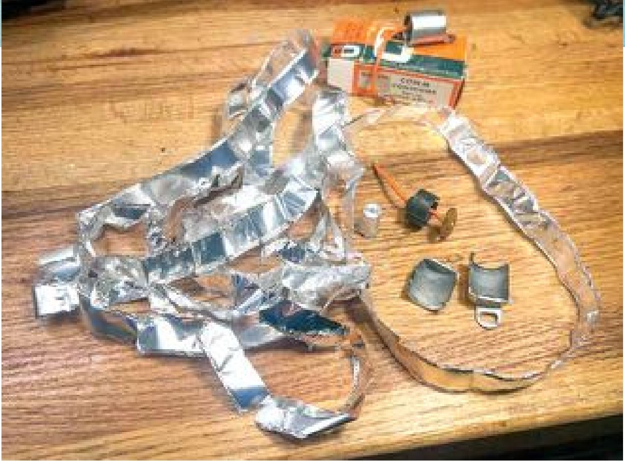
Inside the condenser.
