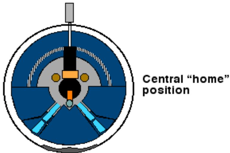
To illustrate how all this works, assume we elect to activate the right turn signal. The spring-loaded piston/wheel at the bottom of the signal arm moves clockwise and presses down on the top of the right turn cam rider. This forces the right signal cam rider outwards and also pushes the piston/wheel into the cam rider slot, holding the arm in the rightmost position. Note that this also compresses right side of the signal arm return spring.
