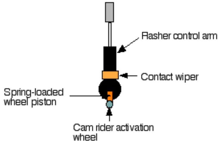
The signal or flasher control arm is equipped with a small spring-loaded square piston on its bottom edge. At the end of this piston is a small metal wheel which provide for smooth operation of the arm and also presses against the inner ends of the cam riders when either the left or right signal is activated. When no signal is activated, this wheel rests in a “V” shaped area between the cam riders.
